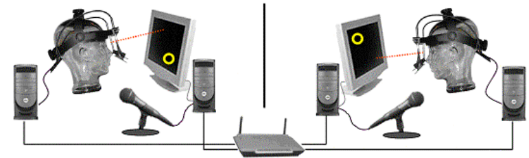
figure 2. The Shared Gaze System (Brennan et al., 2005, 2008). Each person's gaze cursor (yellow circle) is superimposed in real time on the partner's screen. There is an optional voice channel.
