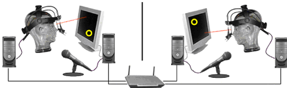
Fig. 1. Schematic of our shared gaze collaborative search system. Searchers were seated in front of identical 19 in. SVGA computer monitors in separate rooms. Synchronized Pentium-based computers outputted displays to each monitor, so that each searcher saw the same stimulus and performed the same search task. Display and eyetracker computers were connected via an Ethernet hub, enabling the bidirectional exchange of gaze signals: the eye position from each searcher's eyetracker could be displayed as a gaze cursor (a 1.7° yellow ring) superimposed over the other's search display. An estimated 24 ms was needed to obtain a fixation position from A and to draw the corresponding gaze cursor on B's monitor, based on a 500 Hz gaze position sampling frequency and a 100 Hz monitor refresh rate.
